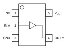
Figure 1. Pinout (Top View)
