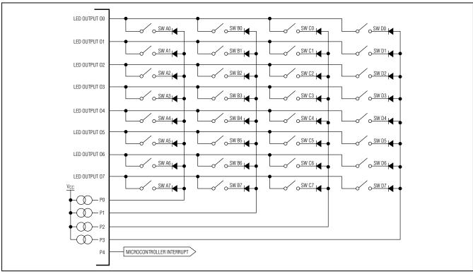
Figure 7. Key-Scanning Configuration
