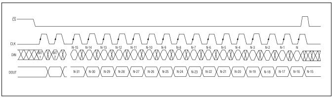
Figure 5. Transmission of More than 16 Bits to the MAX6954
