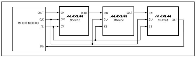
Figure 2. MAX6954 Daisy-Chain Connection
