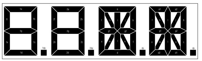
Figure 1. Segment Labeling for 7-Segment Display, 14-Segment Display, and 16-Segment Display
