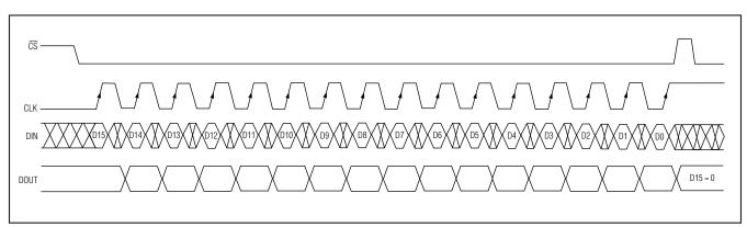
Figure 4. Transmission of 16 Bits to the MAX6954
