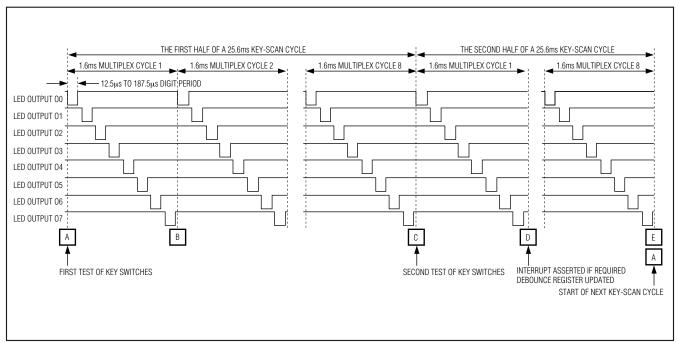
Figure 8. Key-Scan Timing Diagram
