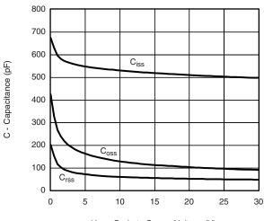
V<sub>DS</sub> - Drain-to-Source Voltage (V) **Capacitance**
