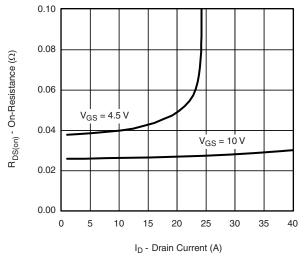
On-Resistance vs. Drain Current
