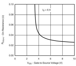
On-Resistance vs. Gate-to-Source Voltage
