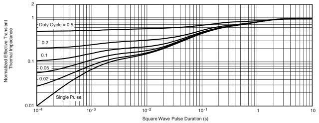
Normalized Thermal Transient Impedance, Junction-to-Foot
