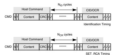
Figure 26. Timing Diagrams at Identification Mode
