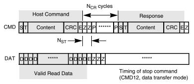
Figure 28. Timing Diagrams at Data Read
