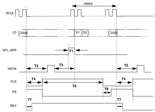
Figure 21. Sharp TFT Panel Timing
