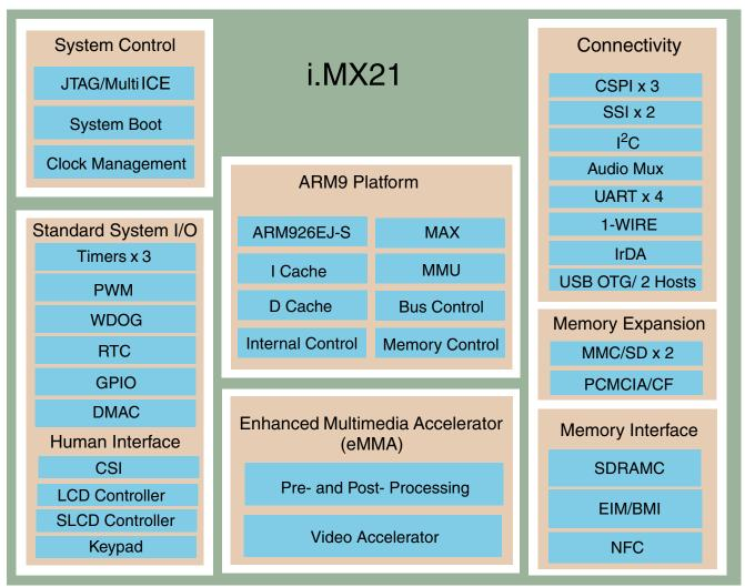
Figure 1. i.MX21 Functional Block Diagram
