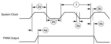
Figure 37. PWM Output Timing Diagram
