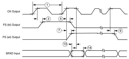
Figure 43. SSI Receiver Internal Clock Timing Diagram
