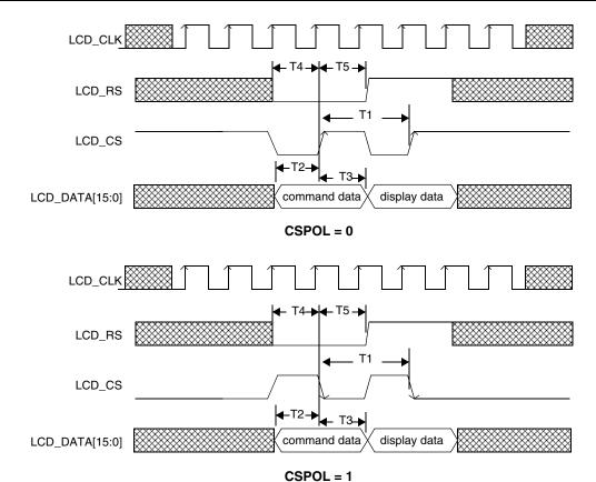
Figure 24. SLCDC Parallel Transfers Timing
