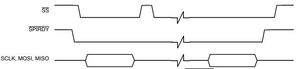
Figure 15. Master CSPI Timing Diagram Using SPI\_RDY Level Trigger
