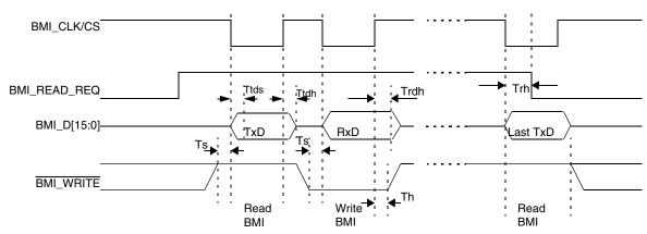
Figure 10. Memory Interface Slave Mode, External Bus Master Read/Write to BMI Timing (MMD MODE SEL=0, MASTER MODE SEL=0)
