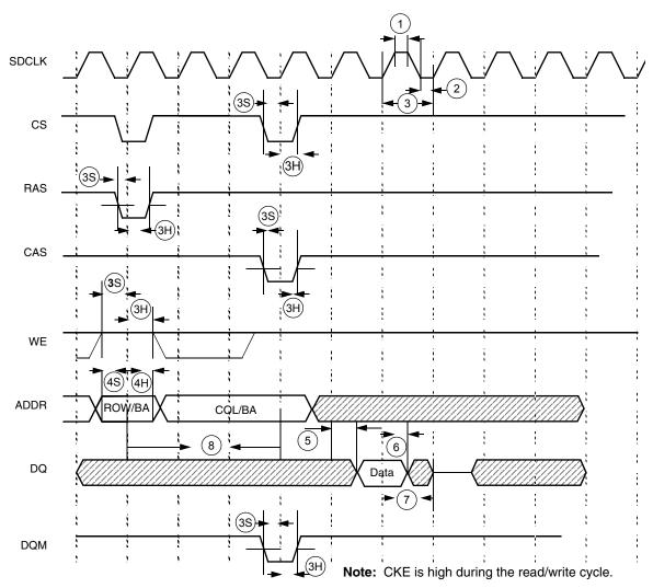
Figure 38. SDRAM Read Cycle Timing Diagram
