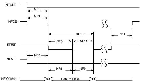
Figure 35. Write Data Latch Timing Dlagram
