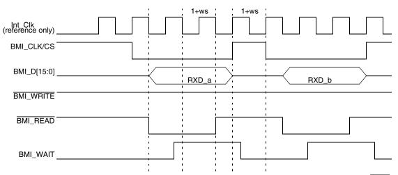
Figure 13. Memory Interface Master Mode, BMI Read to External Slave Device Timing with Wait Signal (MMD\_MODE\_SEL=0, MASTER\_MODE\_SEL=1,WAIT=1)
