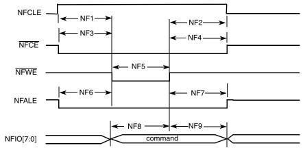
Figure 33. Command Latch Cycle Timing Dlagram
