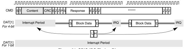
Figure 31. SDIO IRQ Timing Diagram
