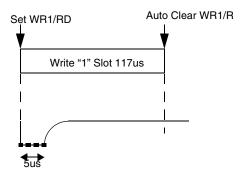
Figure 48. Write 1 Timing
