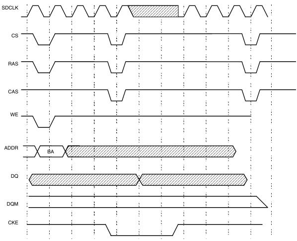
Figure 41. SDRAM Self-Refresh Cycle Timing Diagram
