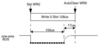
Figure 47. Write 0 Timing
