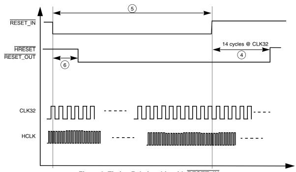
Figure 3. Timing Relationship with RESET\_IN
