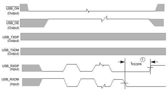
Figure 51. USB Timing Diagram for Data Transfer from USB Transceiver (RX)
