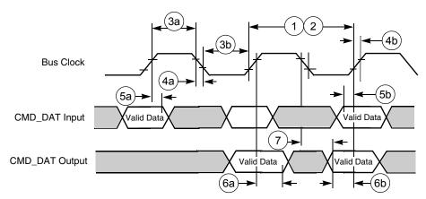
Figure 25. Chip-Select Read Cycle Timing Diagram
