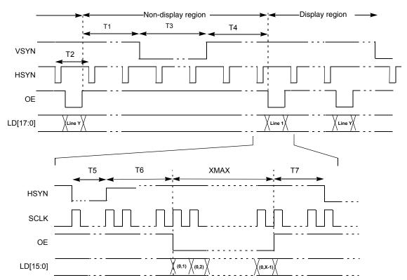
Figure 20. 4/8/12/16/18 Bit/Pixel TFT Color Mode Panel Timing
