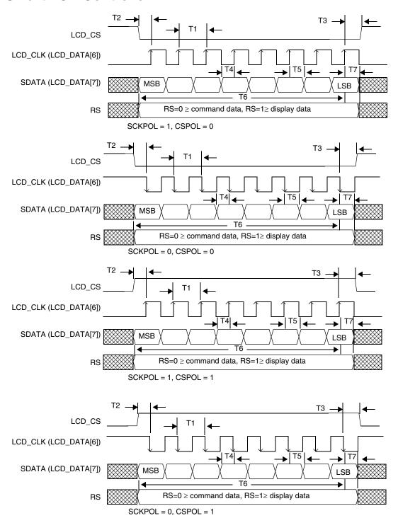
Figure 23. SLCDC Serial Transfer Timing
