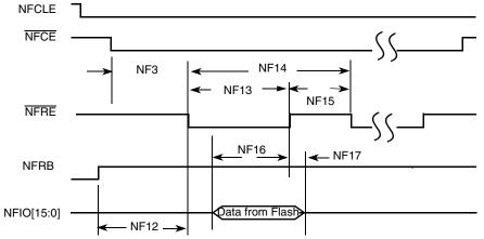
Figure 36. Read Data Latch Timing Diagram
