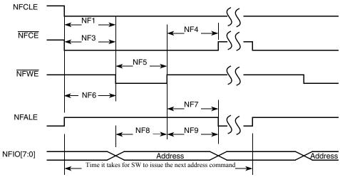
Figure 34. Address Latch Cycle Timing Dlagram
