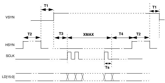
Figure 22. Non-TFT Mode Panel Timing
