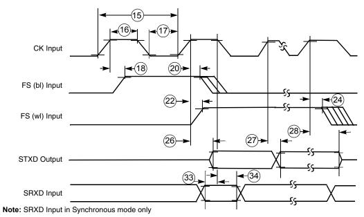
Figure 44. SSI Transmitter External Clock Timing Diagram
