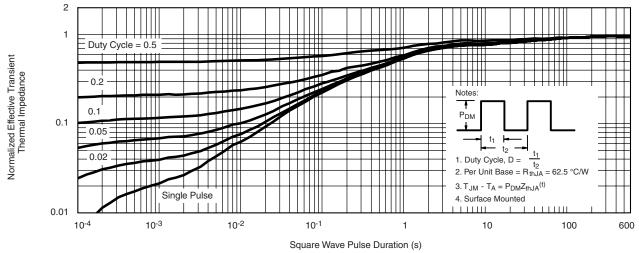
Normalized Thermal Transient Impedance, Junction-to-Ambient
