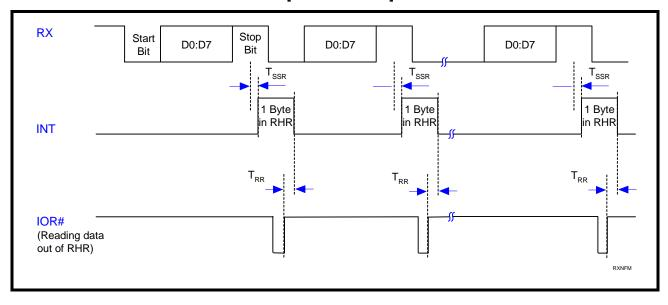
FIGURE 19. TRANSMIT READY INTERRUPT TIMING [NON-FIFO MODE]
