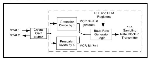
Programming the Baud Rate Generator Registers DLM and DLL provides the capability of selecting the operating data rate. Table 3 shows the standard data rates available with a 14.7456 MHz crystal or external clock at 16X sampling rate clock rate. When using a non-standard data rate crystal or external clock, the divisor value can be calculated for DLL/DLM with the following equation.
