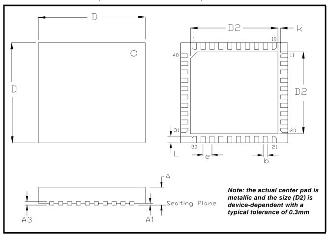
Note: The control dimension is in millimeter.
