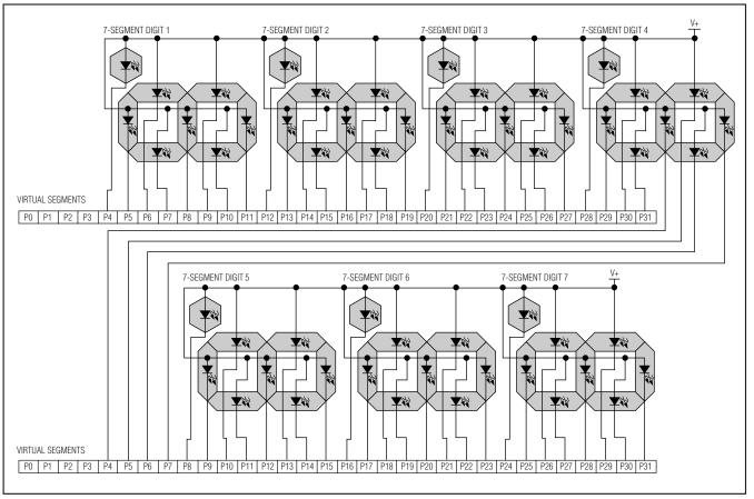
Figure 7. Two MAX6956s Controlling Seven 7-Segment Displays
