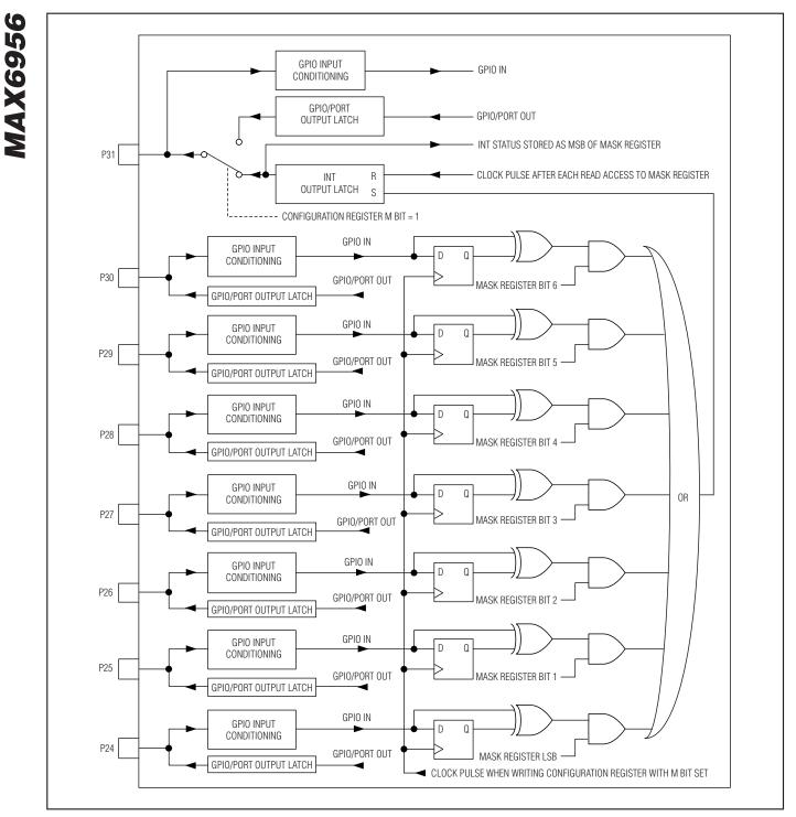
Figure 11. Maskable GPIO Ports P24 Through P31
