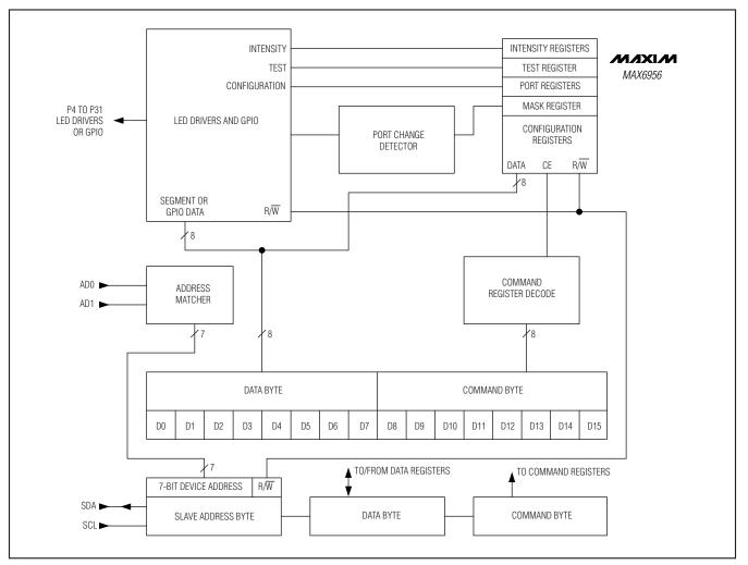
Figure 1. MAX6956 Functional Diagram
