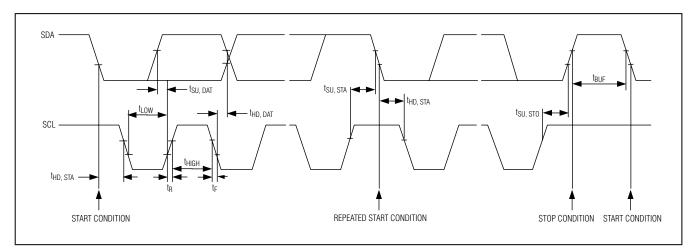
Figure 2. 2-Wire Serial Interface Timing Details
